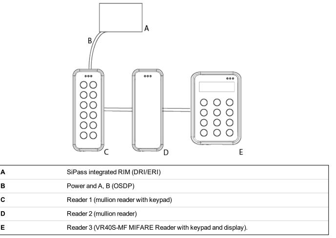
The connection between a reader and a Reader Interface Module (RIM) is as follows:
