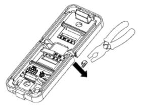
4. Remove the corresponding knockout on the cover.
